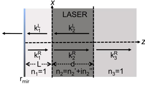
FIG. S2. Schematic of a laser with self-feedback. A mirror of reflectivity  $r_{mir}$  allows light emitted by medium two to be re-injected. The feedback alters the laser threshold, and can be modeled by an effective facet reflectivity  $r_{21}^{\text{eff}}$ , which differs from the bare facet reflectivity  $r_{21}$  in the absence of feedback.
